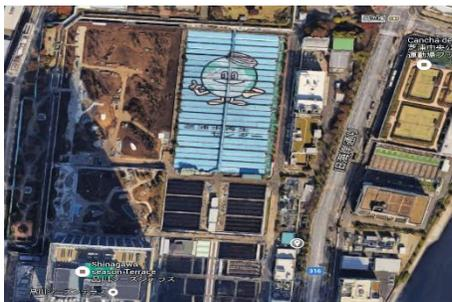
Here ends the treatment, which shows an efficient way of dealing with wastewater in a highly densely populated city, where the lack of space requires these facilities to be installed near commercial areas. The primary and secondary treatment is completely covered, minimizing bad smells. All waste generated is treated, and water is returned to its natural cycle preventing harms for the human health and ecosystem.
